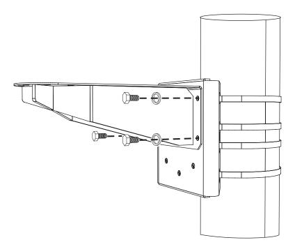
Figure 3. PAXM100 Installation
